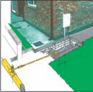
Typical service arrangement
